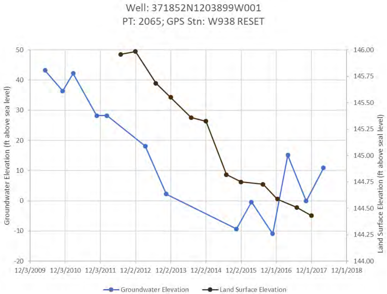
Figure 2-85: Subsidence vs Groundwater Elevation Comparison #2
