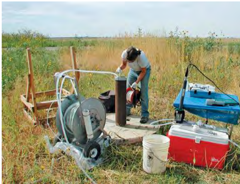
Figure 5 – Typical Groundwater Quality Sampling Event
