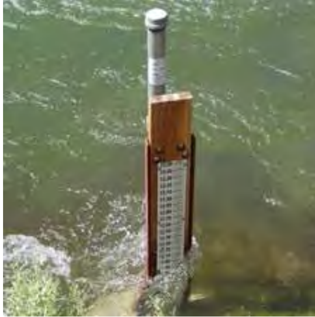
Figure 6 – Simple Stilling Well and Staff Gage Setup
