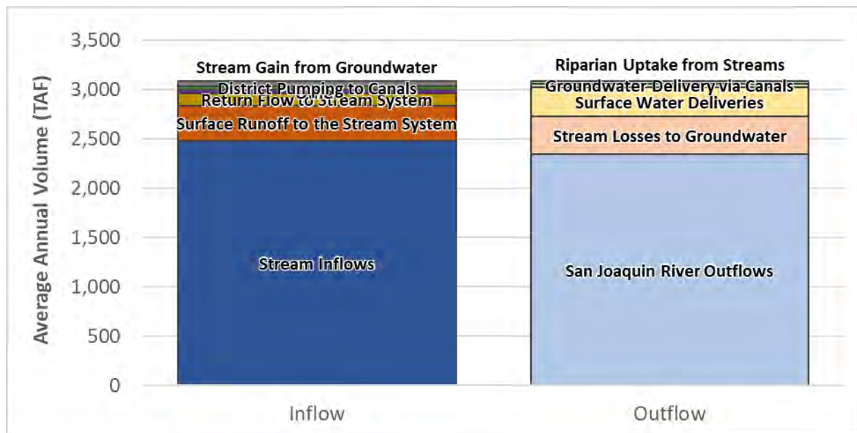
Figure 2-96: Current Conditions Average Annual Water Budget – Stream and Canal Systems, Merced Subbasin
