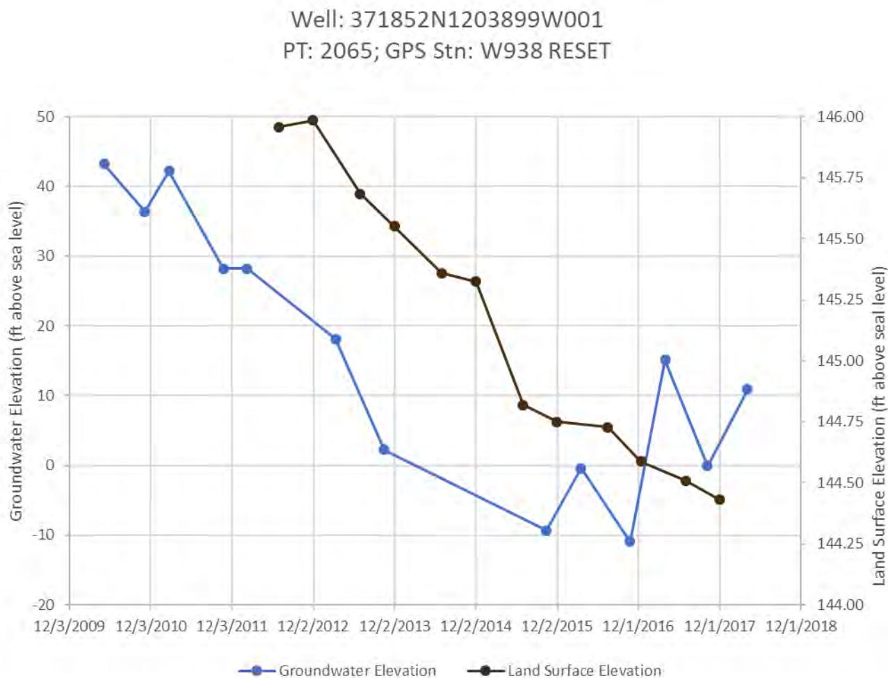
Figure 2-84: Subsidence vs Groundwater Elevation Comparison #2
