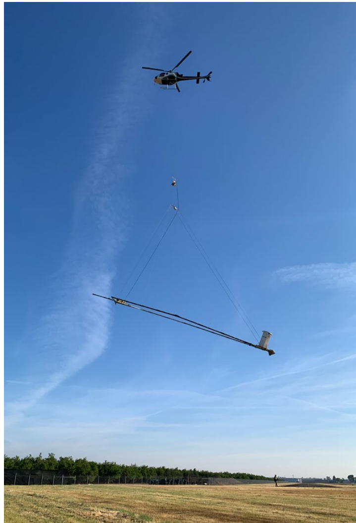
Figure 0-2 Helicopter towing the hexagonal SkyTEM system while collecting AEM data during the survey.
