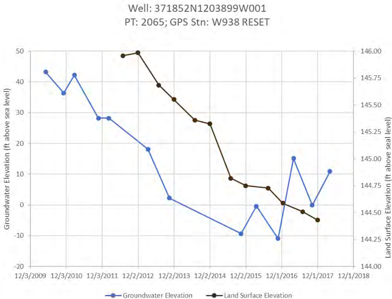
Figure 1-43: Subsidence vs Groundwater Elevation Comparison #2
